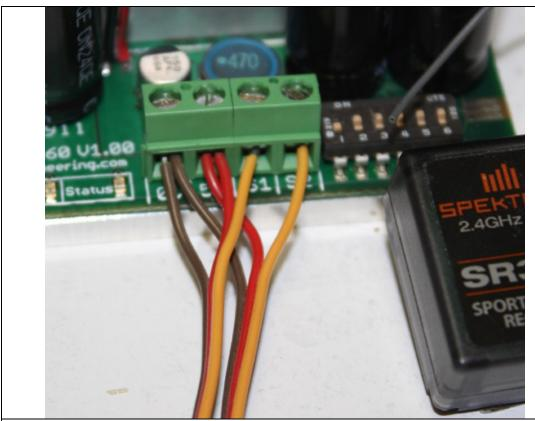
Figure 5.1: R/C connection. Each pigtail is connected to 0V, 5V, and either S1 or S2. An example connection would be the S1 pigtail to elevator and the S2 pigtail to aileron.
