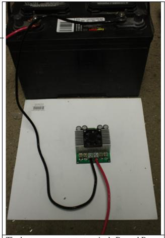
The battery connects to terminals B+ and B-
