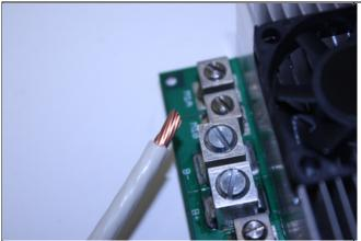
**Step 1:** Strip the wire which you are using approximately <sup>1</sup>/<sub>4</sub>". Use thicker wire for high current applications. *See the chart on the next page for wiring guidelines.*
