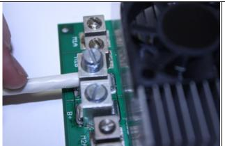
**Step 3:** Insert the stripped portion of the wire into the opening in the screw terminal. Make sure no wire sticks out the other side! Having wire sticking out the other side may contact the heatsink. This could cause a serious short if two wires are allowed to contact the heatsink and power is applied to the unit.
