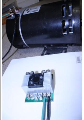
The motors connect to terminals M1A/B and M2A/B
