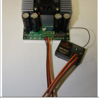
Figure 2.2: R/C input using a receiver powered from terminal 5V
