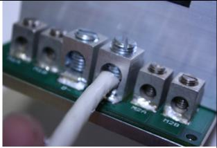
**Step 4:** Turn the top screw clockwise until you encounter resistance, then tighten the screw firmly. Pull on the wire gently to ensure that it is secured.
