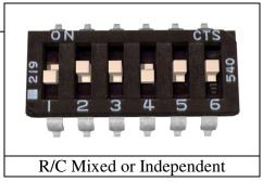
turning of the vehicle. When switch 4 is in the DOWN position, Independent mode is selected. In this mode, the signal fed to the S1 input directly controls Motor 1 (M1A and M1B) and the signal fed to S2 controls Motor 2.
