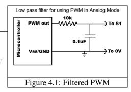
motor operation, at a cost of slower transient response. A PWM frequency higher than 1000Hz is recommended.
