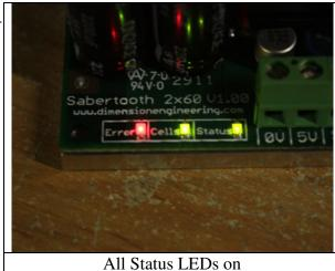
The red Error LED illuminates if the Sabertooth has detected a problem. It will light if the driver has shut down due to a depleted battery or due to overheating, overcurrent or overvoltage. The Error LED will flash along with Cells if there is an issue with your battery. If both of those are blinking simultaneously, your battery is depleted.
