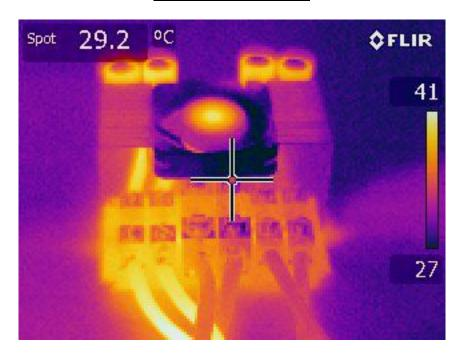
This thermal camera photo was taken with a Sabertooth 2x60 running 40A continuously on both motors. The left side is using 12ga stranded wire. The right side is using 8ga stranded wire. As you can see, the 12ga wire is not only heating itself up due to being undersized, but it is also causing heat to build up in the connections around it.
