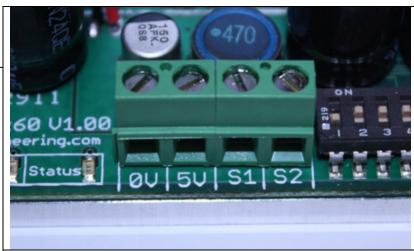
The 5V terminal can be used to power loads up to 1A continuously and 1.5A for peaks. The 0V signal must be connected to the ground of the device generating the input signal.
